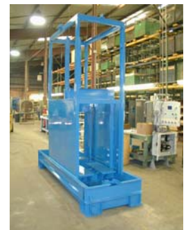
Main Frame Painted after witness test disassembly
