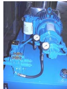
30HP Hydraulic Power Unit
